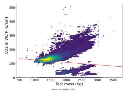
Figure 6: Best linear fitting of the WLTP CO2 emissions for cars registered in 2021, as a function of the test mass of the vehicle
