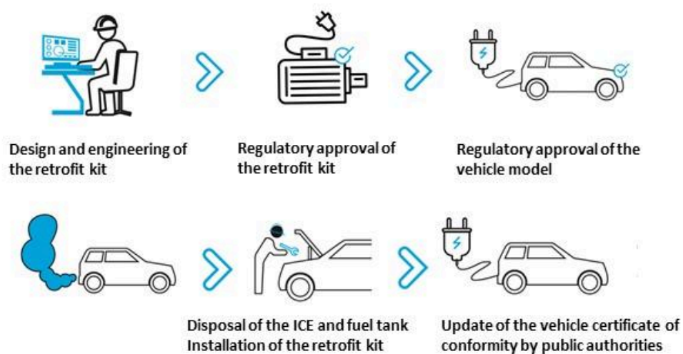
Simplified process for vehicle regulatory approval in France. Source: adapted from Algoé (2020)
