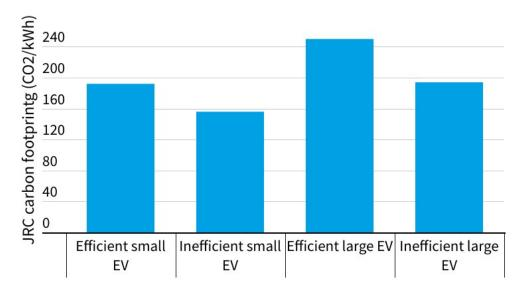
Assumptions: efficient small EV (0.13 kWh/km, 50 kWh battery), inefficient small EV (0.16 kWh/km, 50 kWh), efficient large EV (0.14 kWh/km, 70 kWh), inefficient large EV (0.18 kWh/km, 70 kWh). Carbon footprint of all batteries is 80 kgCO2/kWh (of battery capacity) and total vehicle lifetime is 160,000 km. Metric = total battery carbon footprint (kgCO2) / energy delivered by the EV over its lifetime (kWh)
