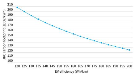
Assumptions: All parameters are kept equal besides the efficiency. Carbon footprint at 80 kgCO2/kWh, battery size 50 kWh, and total vehicle lifetime: 160,000 km. Metric = total battery carbon footprint (kgCO2) / vehicle functional unit (kWh)
