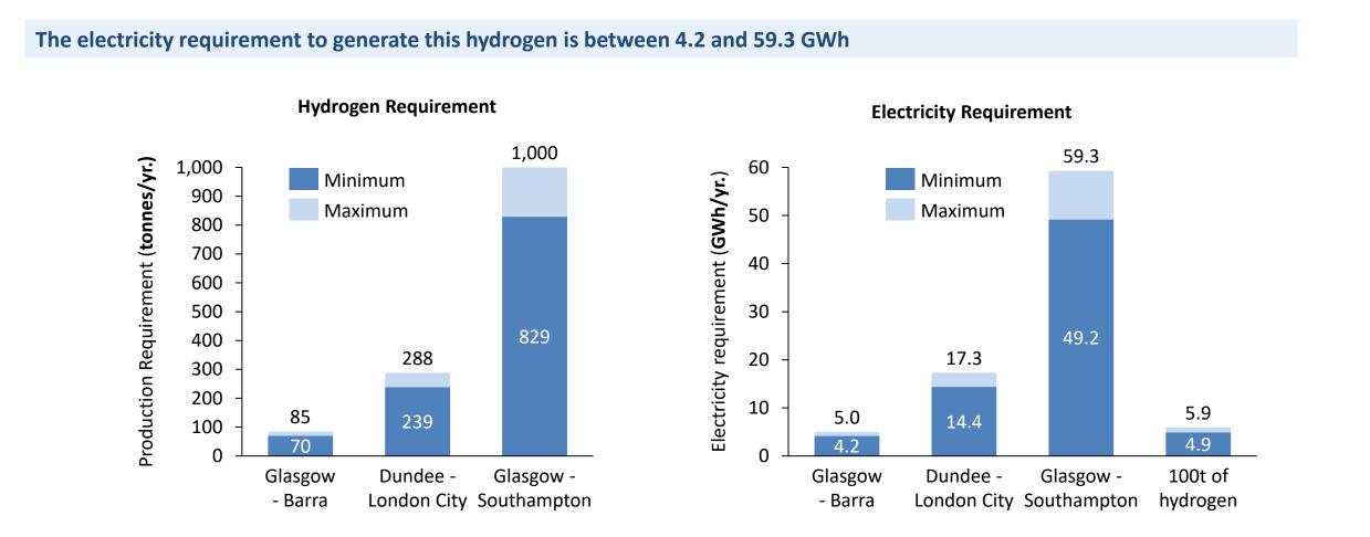
• The values are calculated using the upper and lower bounds for electrolyser efficiency as set out on slide 10
