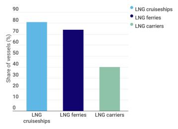
Note: This graph shows the percentage of LNG-powered cruise ships, ferries and LNG carriers that rely on the LNG Otto Dual Fuel Four Stroke Low Pressure Engine. Source: Clarksons Database
