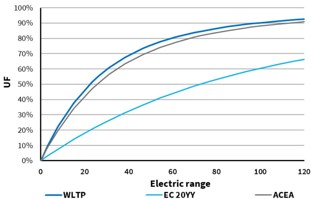
**Figure 3: WLTP and proposed UF curves. EC 20YY is based on dj=2600 and ACEA is based on dj=914.**
