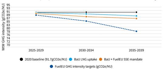
GHG intensity trajectories under BaU, FuelEU's SSE mandate and GHG targets
