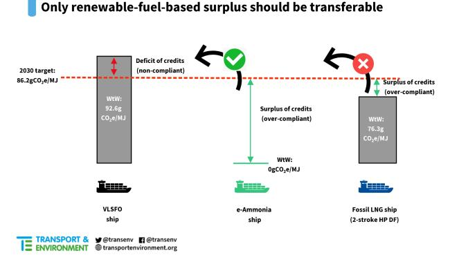
Figure 12: Example of surplus credit exchange limited to ships using RFNBOs (T&E recommendation)
