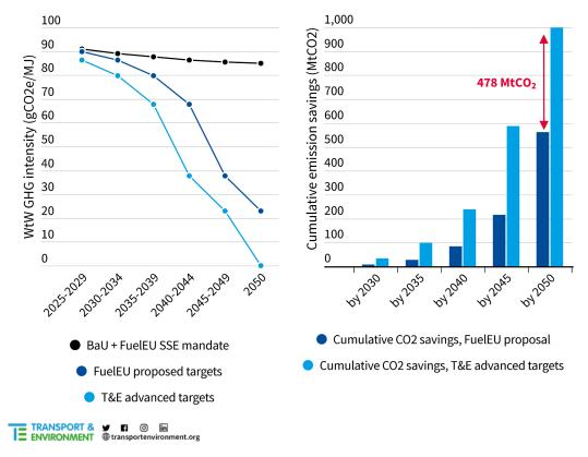
Figure 7: GHG intensity targets proposed in FuelEU and recommended by T&E, and resulting emission savings compared to BaU with only the FuelEU SSE mandate
