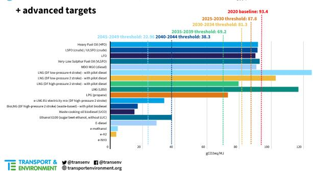
Figure 8: Comparison of WTW GHG intensity of different fuels under different GWP time horizons for methane and FuelEU GHG targets (as proposed or advanced by 5 years)
