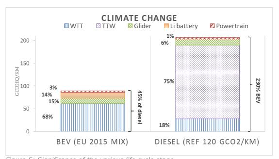
Figure 5: Significance of the various life cycle stage The basic assumptions are: a life time driven distance of 2
