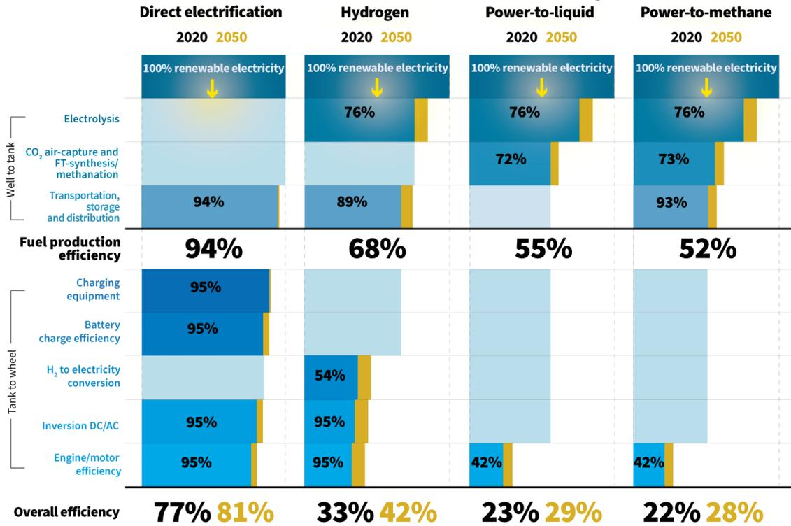
Notes: Efficiency rates of long-haul HGVs. To be understood as approximate mean values taking into account different production methods. Direct electrification represents both BEVs running on batteries and/or overhead catenaries. Hydrogen includes onboard fuel compression, while power-to-methane includes fuel liquefaction. Assuming same engine efficiency for diesel and dual-fuel HPDI gas vehicles. Excluding mechanical losses.
