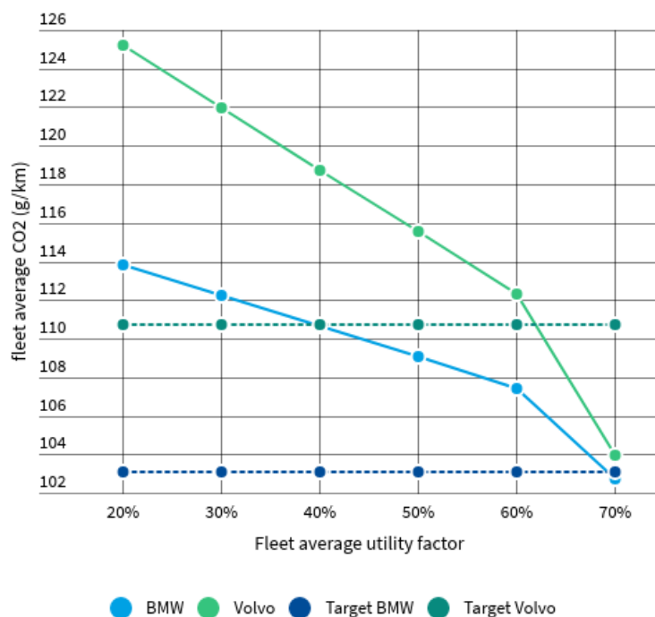
Figure 3: Impact of PHEV fleet average utility factors (share of electric kilometers driven) on fleet average CO2 emissions of BMW and Volvo.
