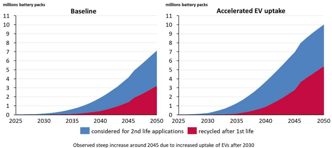
Figure 6: Fate of recovered batteries (million battery packs per annum)
