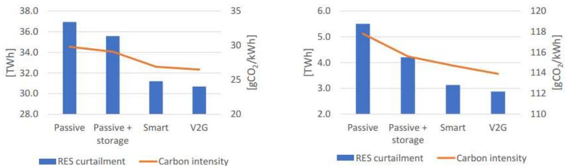
Figure 16: Curtailment and grid averaged CO<sub>2</sub> reduction: FR (left); IT (right)
