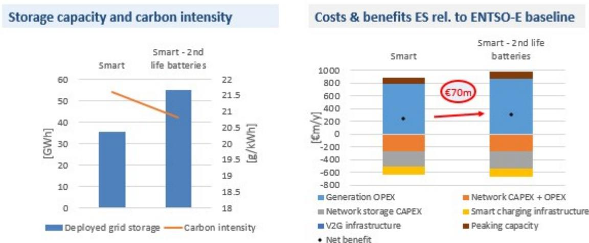
Figure 21: storage capacity and carbon intensity (left) and system costs and benefits in the Smart scenario in Spain with new batteries and 2nd life batteries (right)
