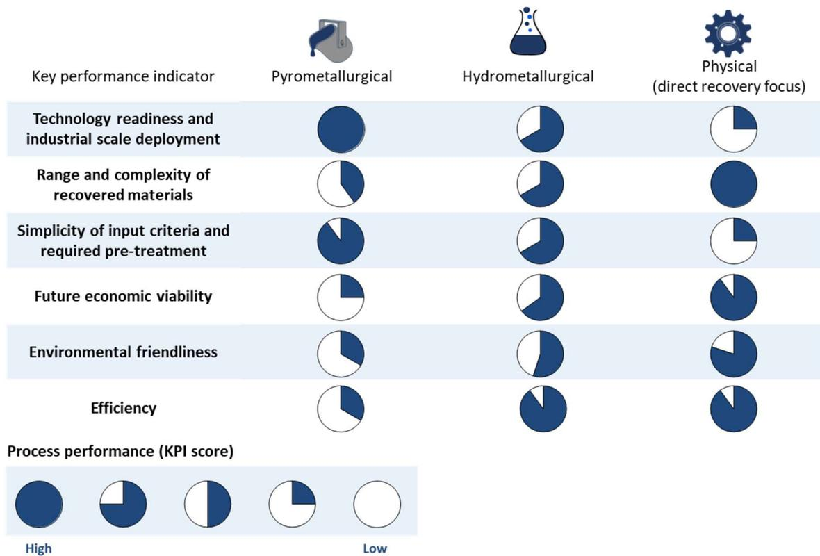
Figure 25: Qualitative comparison of recycling processes (2019Q1)
