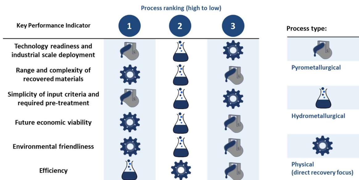
**Figure 38: Summary of assessment of battery recycling processes (ranking of performance against KPIs shown in section 4.2, 1 = high, 3 = low)**
