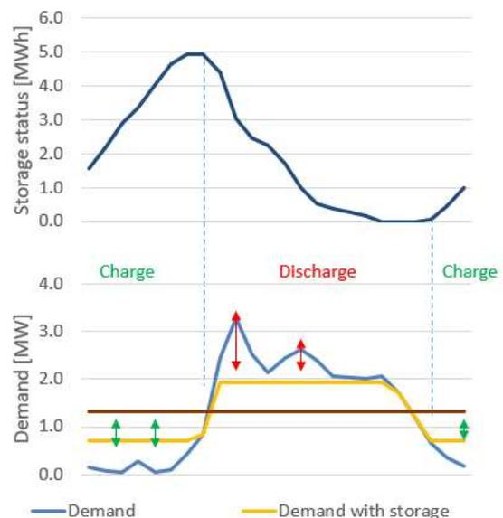
Figure 35: Daily operation of distribution support battery
