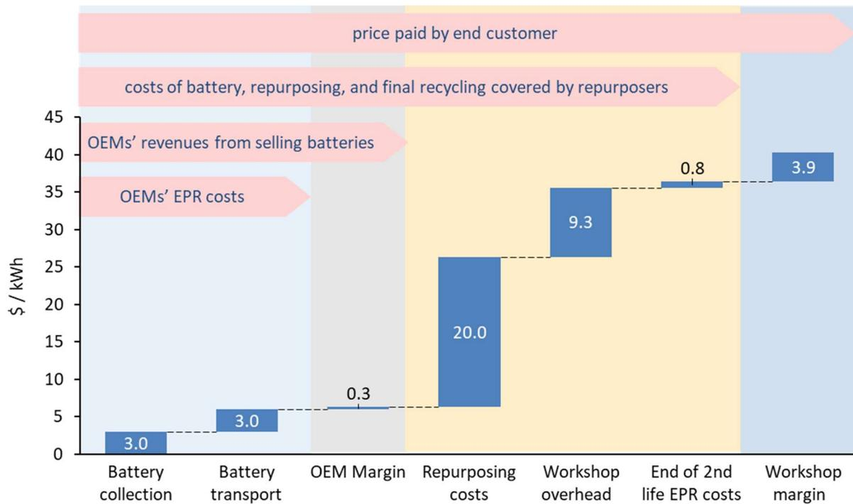
**Figure 33: Price breakdown of a repurposed battery placed on market in 2030<sup>27</sup> (business model based on and validated by industry)**
