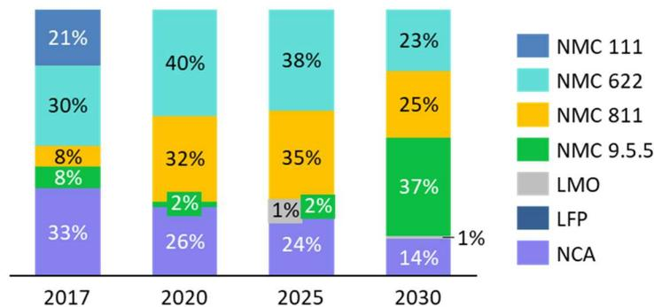
Figure 5: Demand of EV batteries by chemistry in Europe<sup>10</sup>
