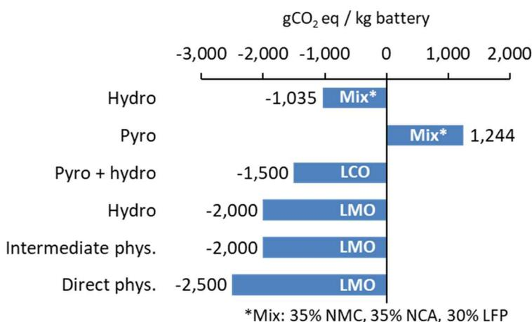
**Figure 24: Comparison of emissions associated with recycling of different LIB chemistries and includes emissions associated with required chemicals for the hydrometallurgical process. Negative values are emissions avoided in the manufacturing of recovered materials thanks to battery recycling**
