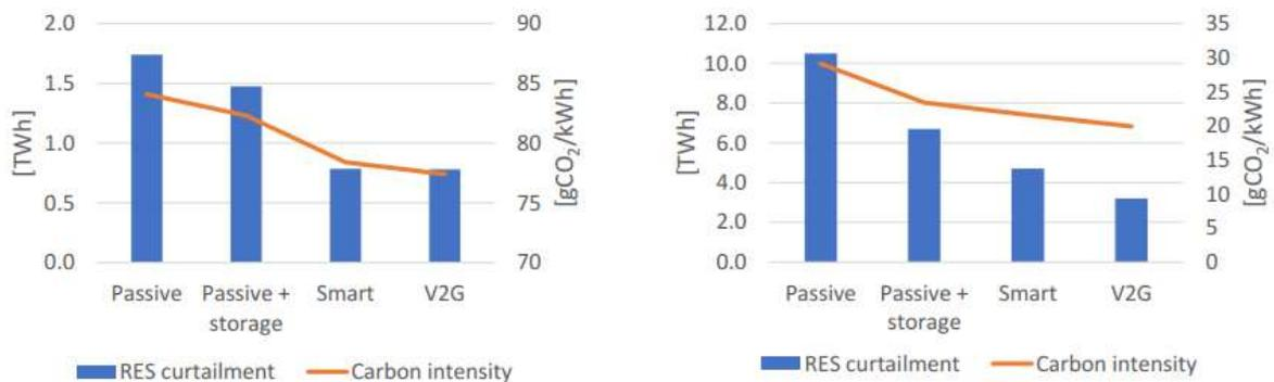
Figure 15: Curtailment and grid averaged CO<sub>2</sub> reduction: GB (left); ES (right)
