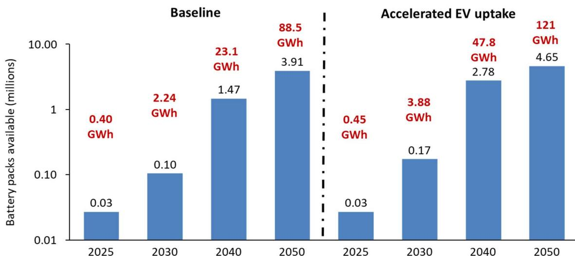
Figure 7: Number of EV battery packs viable for second life applications (bar chart, log scale) and total residual capacity becoming available in key years (GWh per annum)
