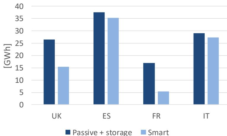
Figure 19: interaction between grid batteries and smart demand (2040)
