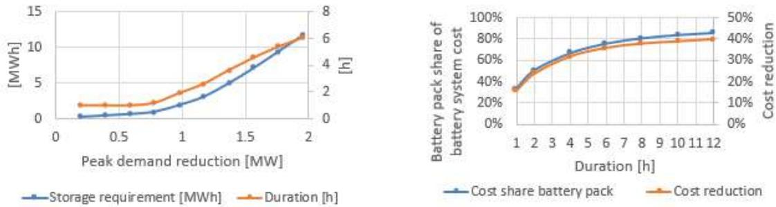
Figure 36: Left: Impact of battery storage capacity on peak demand reduction. Right: trade off with larger batteries and the impact of 2<sup>nd</sup> life costs.
