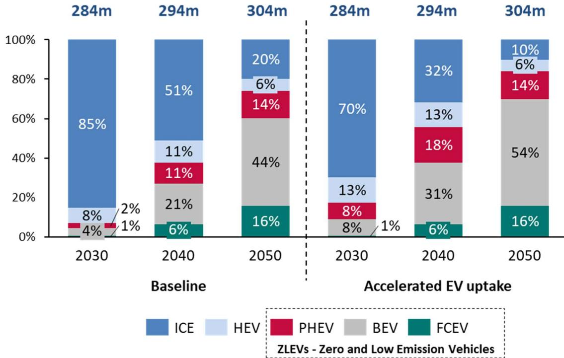
**Figure 2: Structure of the European vehicle stock by powertrain in two key years (figures on top of stacks refer to the absolute EU car stock size)**
