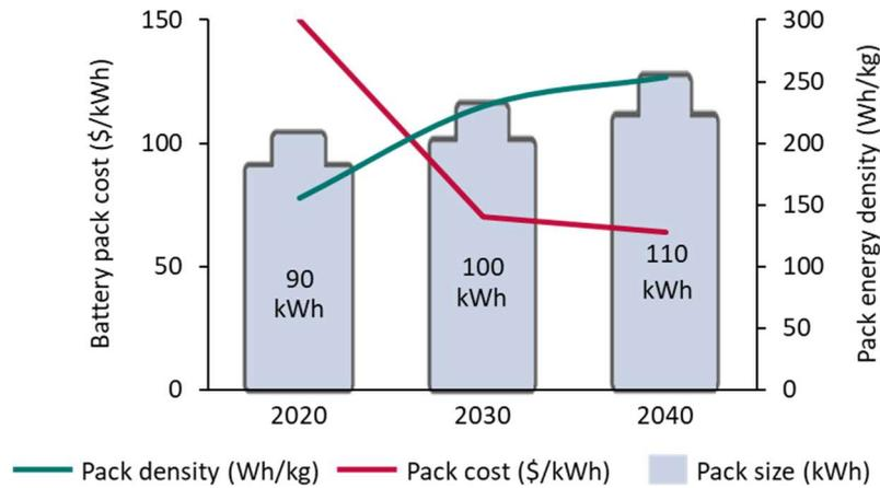
Figure 4: Key features of future batteries deployed in large size BEVs<sup>9</sup>
