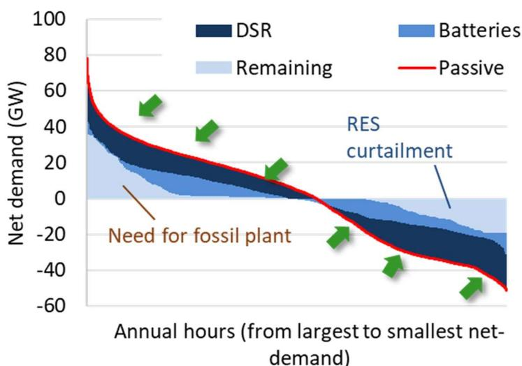
Figure 10 Example annual net load for a decarbonised power system
