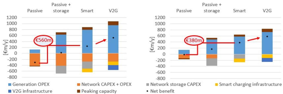
Figure 18: Whole system cost and benefits 2040 in Spain: with original EV charging pattern (left) and with higher daytime charging ratio (right)
