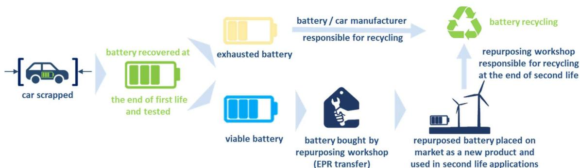
**Figure 27: Potential business and EPR transfer model for EV batteries**
