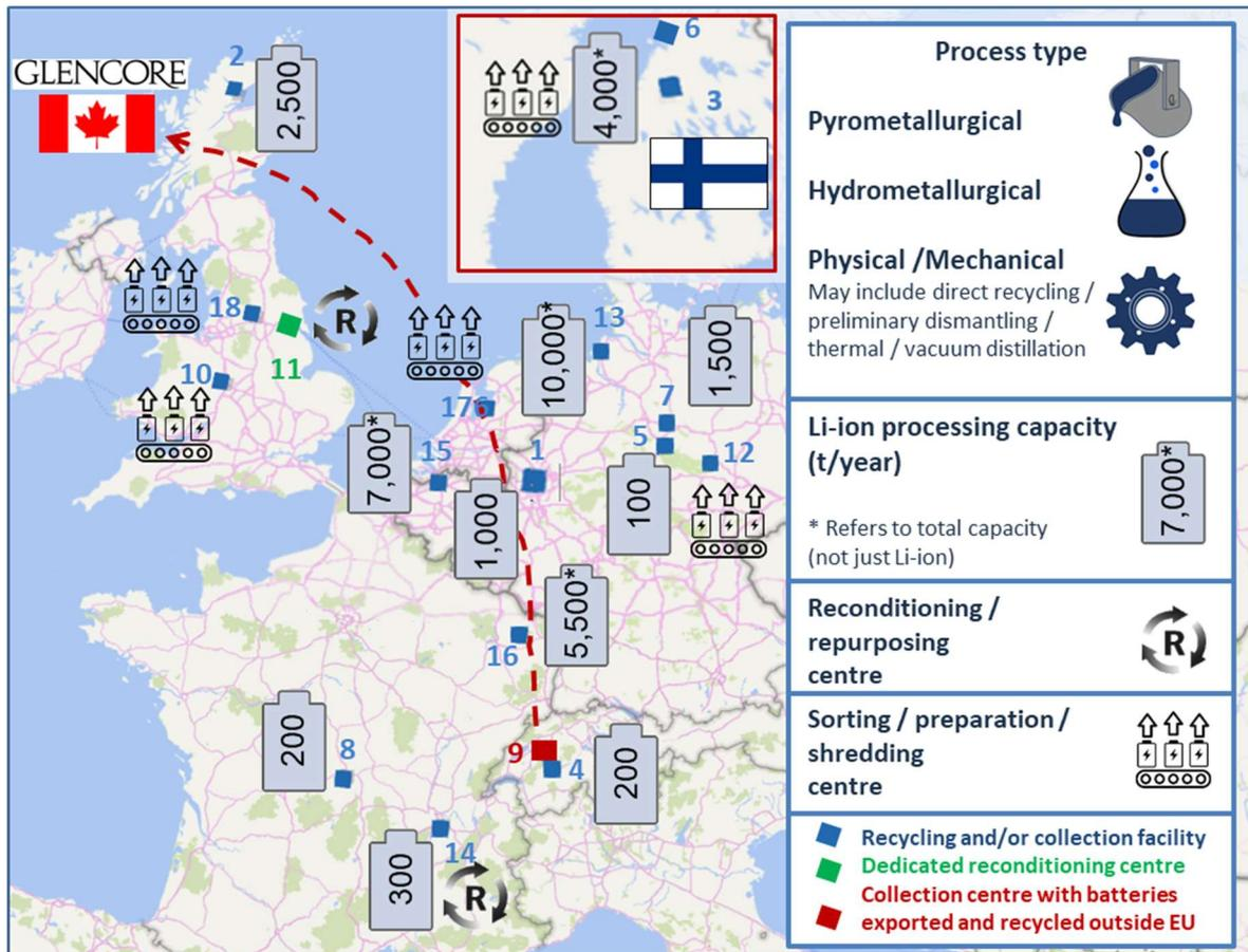
Figure 26: Overview of facilities processing and recycling Li-ion batteries in Europe (2018) based on publicly available data collated by Element Energy (capabilities shown in Table 1)
