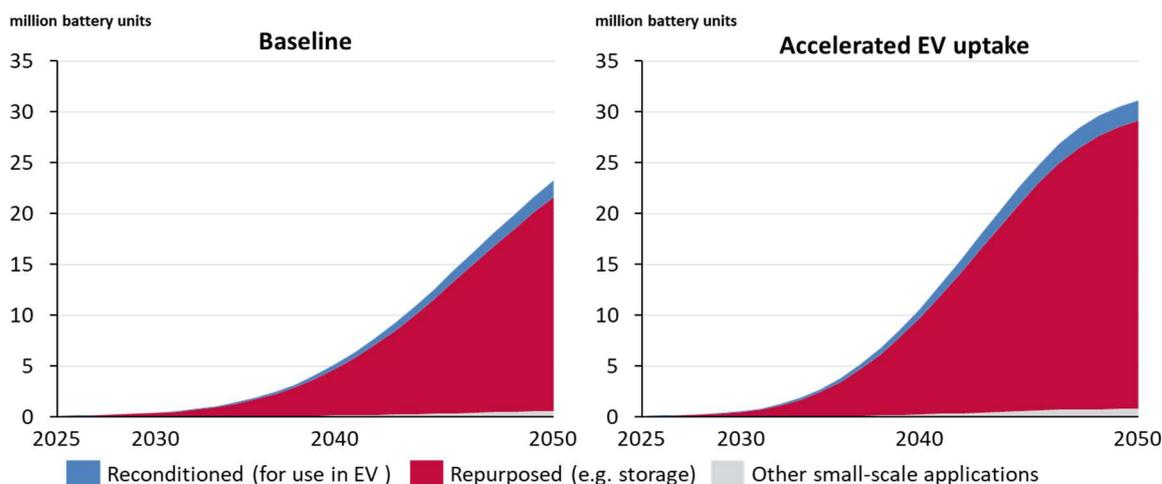
**Figure 8: Structure of the second life battery stock (million units)**
