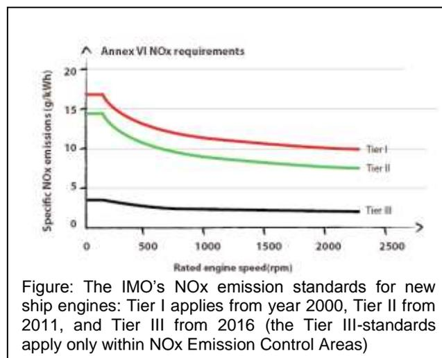
Figure: The IMO's NOx emission standards for new ship engines: Tier I applies from year 2000, Tier II from 2011, and Tier III from 2016 (the Tier III-standards apply only within NOx Emission Control Areas)
