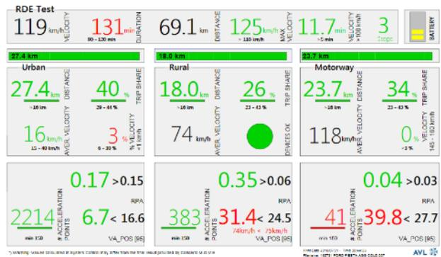
Figure 105: Driving dynamics of segment B vehicle (31/07/2018, non-compliant, extended conditions, cold)
