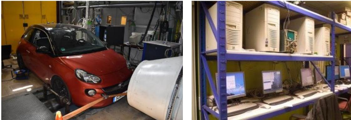
**Figure 5:** LAT chassis dyno (left) and chassis dyno control station (right)
