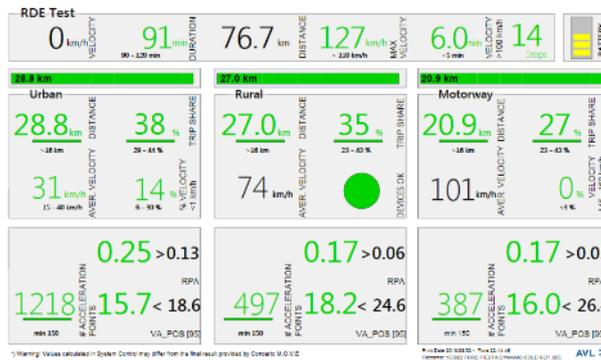
**Figure 130:** Driving dynamics of segment B vehicle (02/08/2018, compliant, dynamic, cold)
