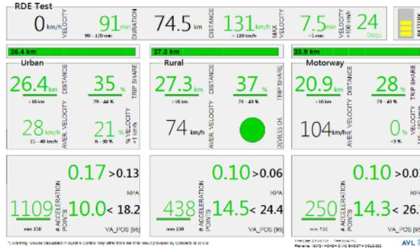
**Figure 84:** Driving dynamics of segment C vehicle (21/07/2018, compliant, smooth, cold)
