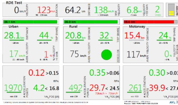
**Figure 118:** Driving dynamics of segment B vehicle (01/08/2018, non-compliant, extended conditions, cold)
