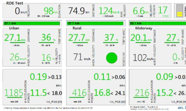
**Figure 112:** Driving dynamics of segment B vehicle (01/08/2018, compliant, smooth, cold)
