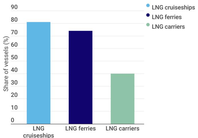
Note: This graph shows the percentage of LNG-powered cruise ships, ferries and LNG carriers that rely on the LNG Otto Dual Fuel Four Stroke Low Pressure Engine. Source: Clarksons Database
