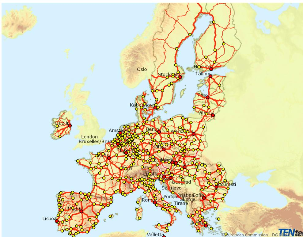
Figure 1<sup>3</sup>: TEN-T core and comprehensive network (bold red: core, yellow: urban nodes)
