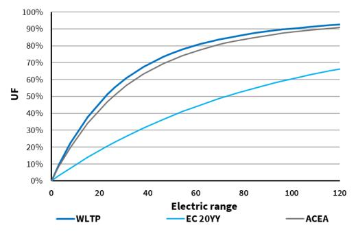
Figure 3: WLTP and proposed UF curves. EC 20YY is based on dj=2600 and ACEA is based on dj=914.
