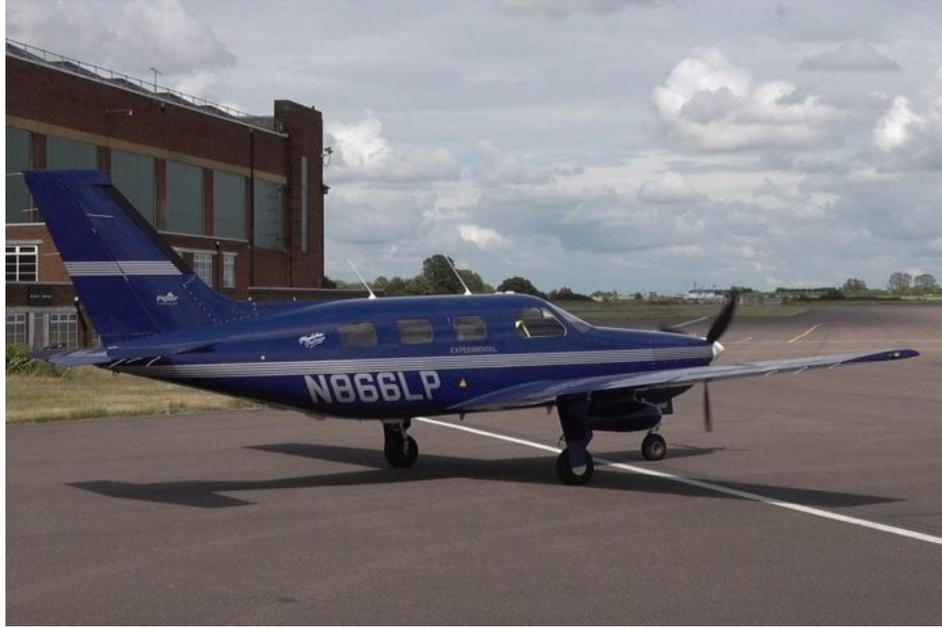
**Figure 12: ZeroAvia's hydrogen fuel cell aircraft, to be commercialized in 2023. Photo: ZeroAvia.**
