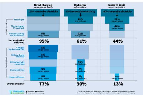
Figure 3: Efficiency of different passenger cars technology pathways based on renewable electricity.<sup>19</sup>
