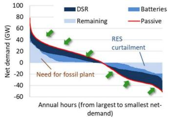
Figure 1: Figure 1: Example annual net load for a decarbonised power system
