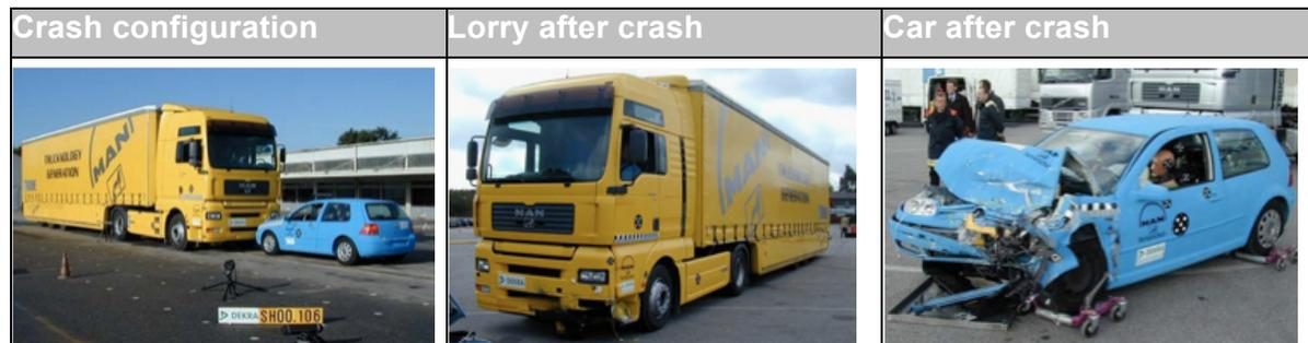
**Figure 4:** crash simulation: lorry speed 21km/h; car speed 42km/h
