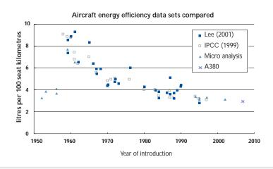
Note that aircraft manufactured in the early 1950s – such as the Lockheed Constellation – were two to three times as fuelefficient as the early jets that succeeded them and virtually as fuel-efficient as the aircraft on sale today.
