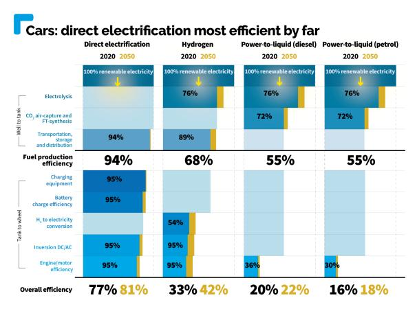
Notes: To be understood as approximate mean values taking into account different production methods. Hydrogen includes onboard fuel compression. Excluding mechanical losses.
