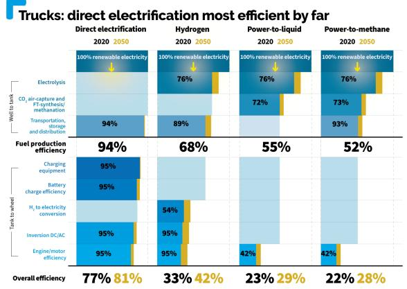
Notes: Efficiency rates of long-haul HGVs. To be understood as approximate mean values taking into account different production methods. Direct electrification represents both BEVs running on batteries and/or overhead catenaries. Hydrogen includes onboard fuel compression, while power-to-methane includes fuel liquefaction. Assuming same engine efficiency for diesel and dual-fuel HPDI gas vehicles. Excluding mechanical losses.
