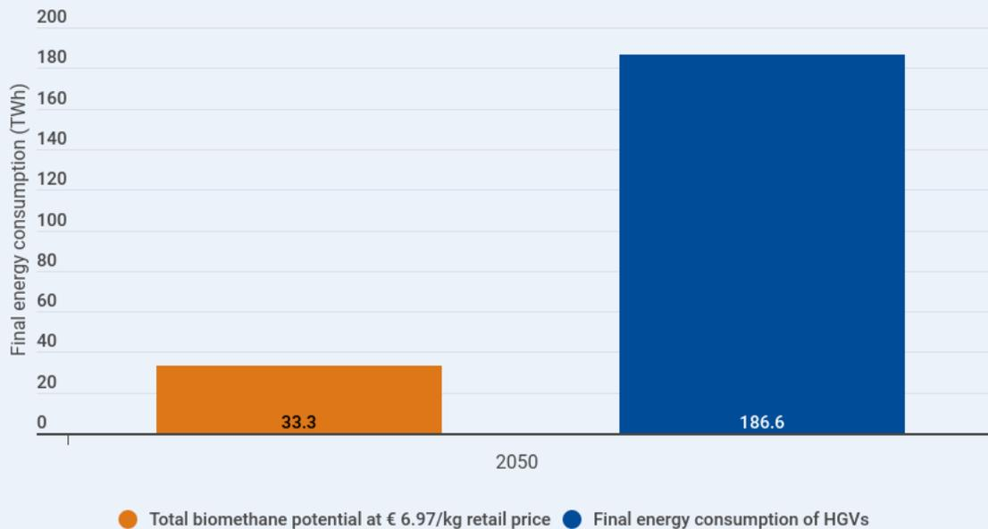
**Notes:** Comparing the final energy consumption of a dual-fuel CI HPDI gas vehicle fleet with the total sustainable biomethane production potential in Germany. Assuming that all available biomethane is supplied to HGVs, leaving nothing for the power, industry or buildings sectors. Based on a biomethane retail price of € 6.79/kg, this is more than six times the average price level of compressed fossil methane (CNG) as a transport fuel in Germany.
