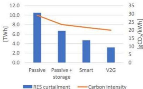
Figure 2: Curtailment and grid averaged CO<sub>2</sub> reduction in Spain
