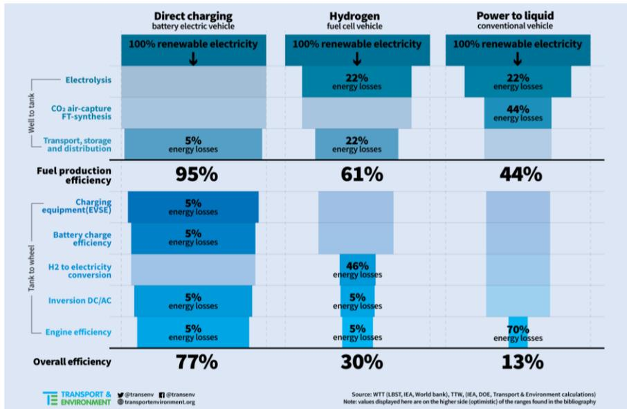
Figure 3: Efficiency of different passenger cars technology pathways based on renewable electricity.<sup>19</sup>
