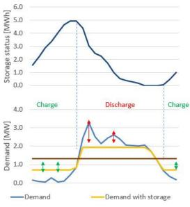
Figure 35: Daily operation of distribution support battery
