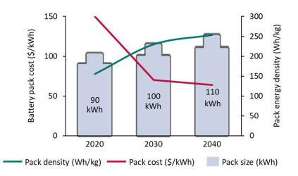
Figure 4: Key features of future batteries deployed in large size BEVs<sup>9</sup>
