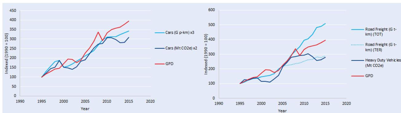
Figure 3: Evolution of Polish GDP, transport activity and emissions. Note that the car passenger activity has been scaled with a factor of 3, car emissions with a factor of 2, to aid visual comparison.
