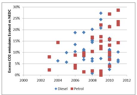
Figure A2.3: Comparison of real-world and test data for selected car models 2003 – 11<sup>6</sup>
