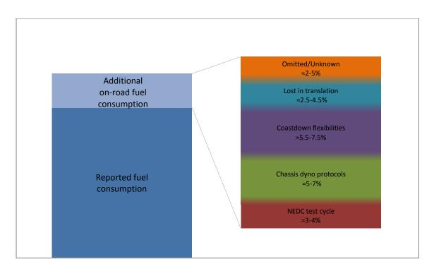
Figure 11: Schematic of causes of the gap between official test and real-world CO<sub>2</sub> emissions
