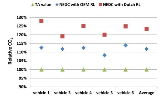
**Figure 9:** Summary NEDC CO<sub>2</sub> emissions of Euro 5 and 6 vehicles with different road load settings (TNO, 2012b)
