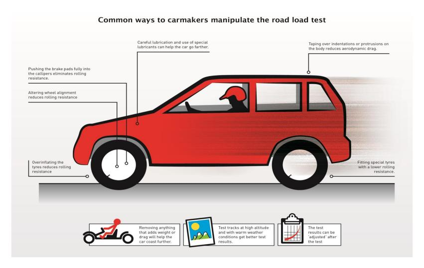
Figure 7: Specific manipulations of the road load test
