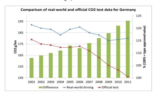
**Figure 2:** Comparison of average real world and official test results for Germany (derived from Mock *et al*, 2012)
