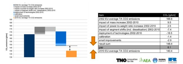
Figure 10: Top-down deployment of the contribution of technologies to CO<sub>2</sub> emissions reductions 2002-10 (TNO, 2012a)
