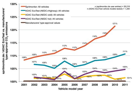
Figure A2.4: Differences in the level of CO<sub>2</sub> emissions from other data sources as percentage of type-approval values over time
