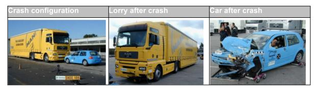
Figure 4: crash simulation: lorry speed 21km/h; car speed 42km/h
